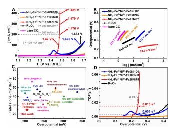
Figure 3. A) Linear sweep voltammetry (LSV) curves and B) Tafel slopes of different materials. C) Comparison of OER overpotential (10 mA cm<sup>-2</sup>) and Tafel slope of NH<sub>3</sub>-Fe<sup>2+</sup>Ni<sup>2+</sup>-Fe25Ni75 with reported catalysts. D) TOF of different materials.
